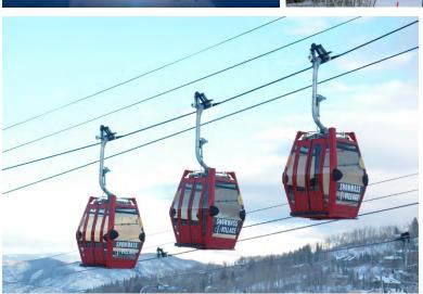
Pulse gondolas have trains with one, two or three cabins per train, and up to six trains that are evenly spaced along the rope. The cabins are fixed to the transport cable. The entire system slows for loading and unloading when the cabins are in the terminals.
